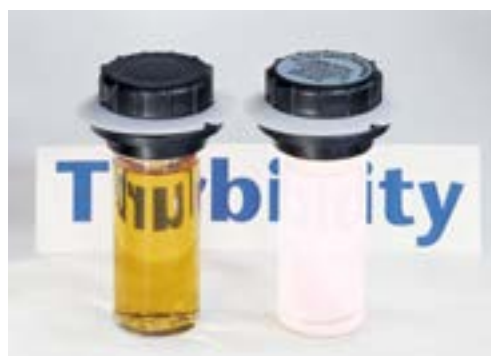
Turbidity measuring cuvette and standard cuvette
